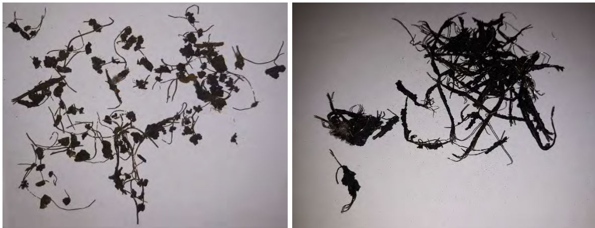
Fig. 5 Agglomerations of rubber and steel wire
