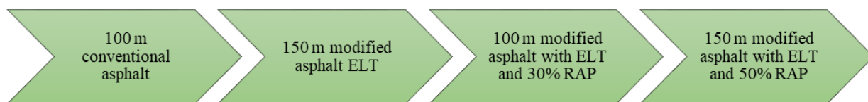
Figure 2. The road sections of total 500 m new asphalt pavement.
