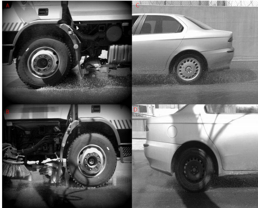
Figure 7. Comparison of heavy truck and passenger car splash and spray photo frames. A) new conventional pavement and B) asphalt mixture with ELTs and 30 % RAP, C) new conventional pavement and D) asphalt mixture with ELTs and 30 % RAP.
